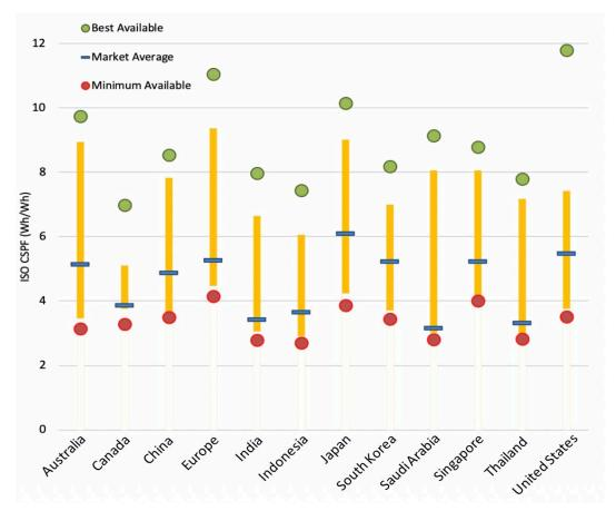
**Figure 3.2: Efficiency of available residential ACs in selected countries/regions.** Efficiency estimated in ISO Cooling Seasonal Performance Factor (CSPF) based on IEA data converted to common metric using relationships in Park et al. (2020). 185
