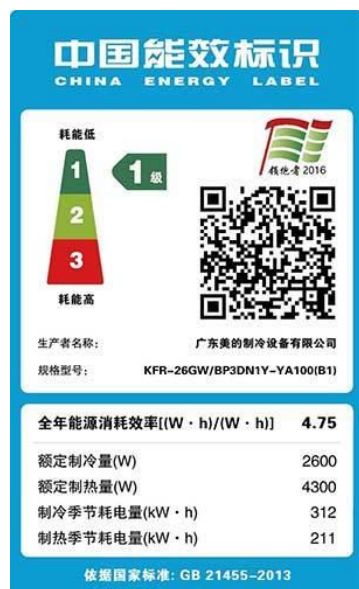
Fig. 12. The China Energy Label includes categories, the "Top Runner" endorsement, and a QR code that enables additional, customized information to be provided to consumers.
